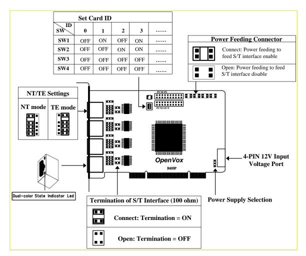
**Figure 3 Jumper setting**
