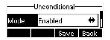
Figure 63 - Activate Call Forward and configure Call Forward Number
