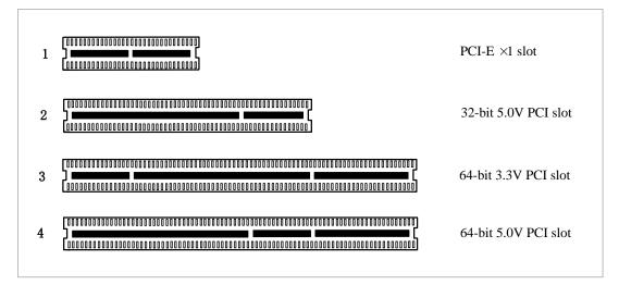
Figure 2 PCI-E and PCI slot
