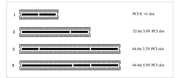
Figure 2 PCI-E and PCI slots
