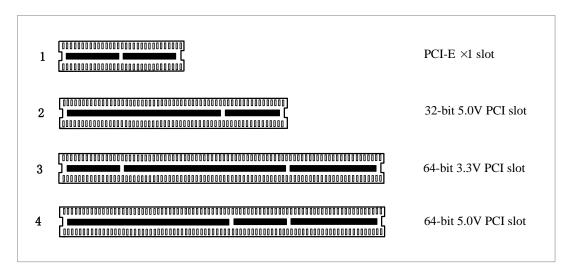
Figure 2 PCI-E and PCI slots
