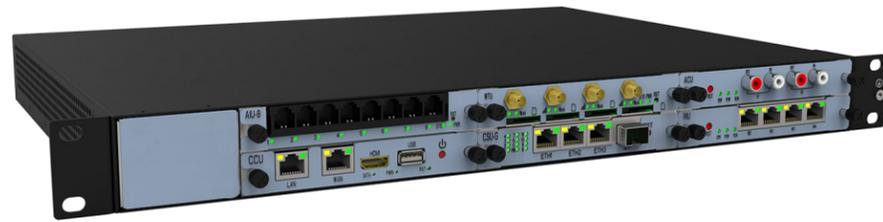
UCP1600 adopts 1U standard chassis, 434mm wide, 330mm deep and 44mm high, which can be installed in a 19-inch cabinet conforming to IEC (International Electrotechnical Commission) standard.
