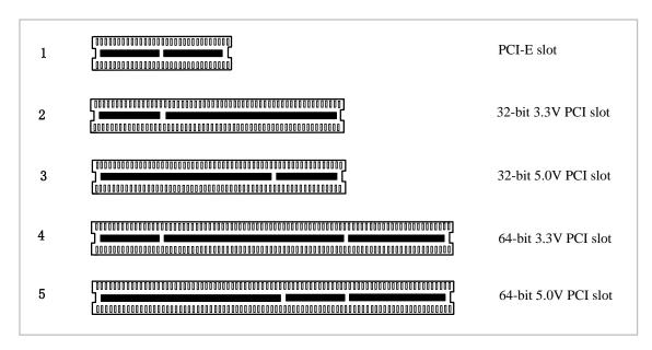
Figure 2 PCI-E and PCI slots
