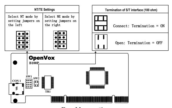
Figure 3 Jumper setting
