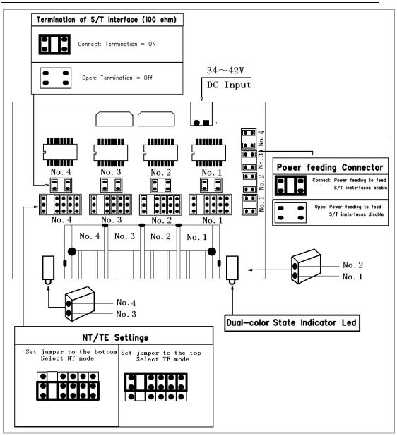
**Figure 5 Jumper Setting**
