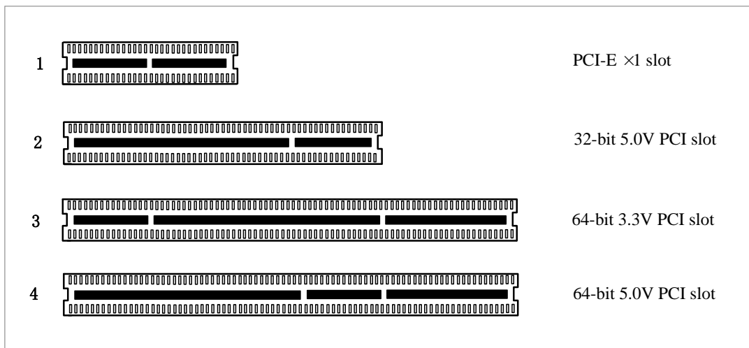
Figure 2 PCI-E and PCI slot
