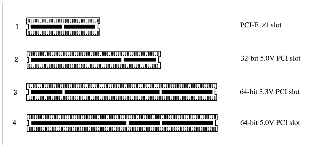
Figure 2 PCI-E and PCI slots
