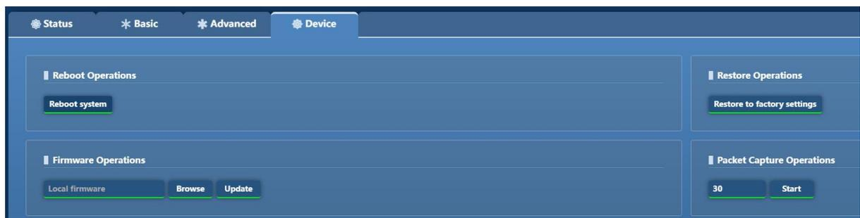
**Restore factory settings:** Clicking the <Restore> button will restore the Wireless Trunked Gateway configuration to factory settings, but will not affect the system IP address related information.
