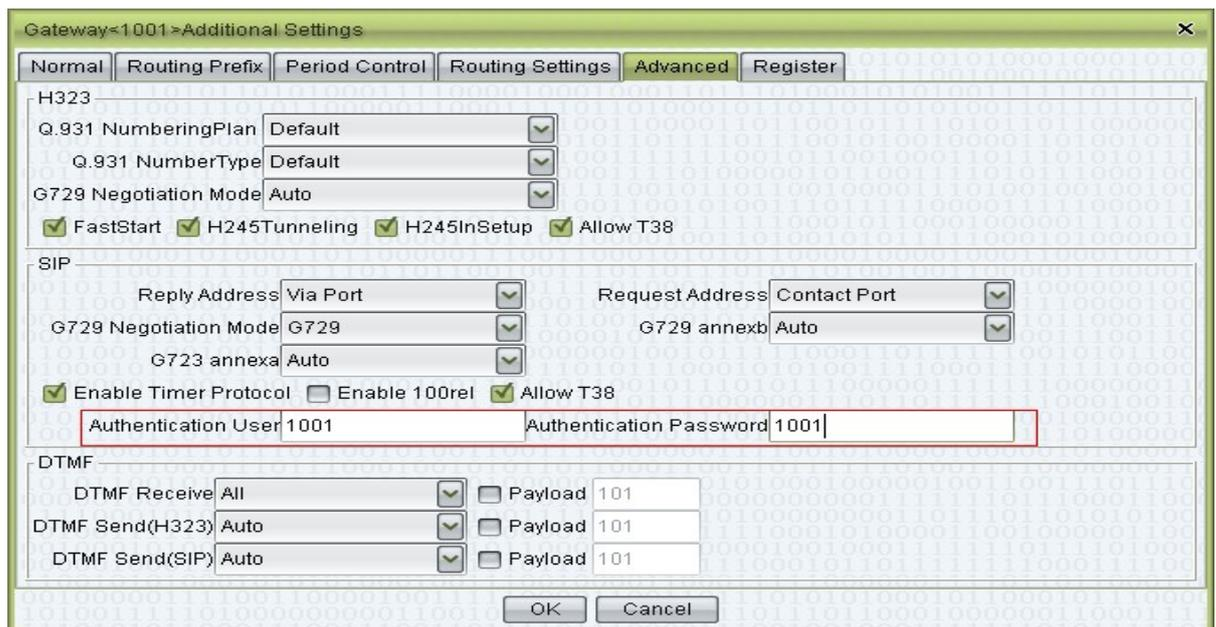
When Register enabled, Authentication User and Password must be filled in.
