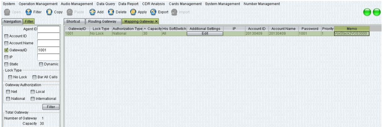
Gateway ID:1001 -----Username of SIP trunk which GSM gateway registers to
