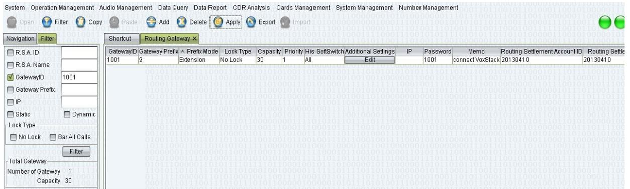
Gateway ID:1001 -----Username of SIP trunk which GSM gateway registers to
