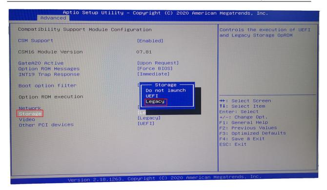
Figure 1-2 CSM configuration
