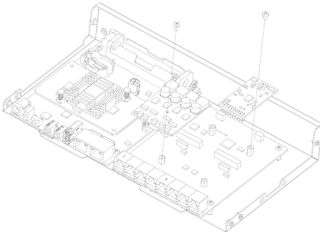
4. After installing the module, insert the chassis vertically as the picture shows, fasten it to the upper case, and then tighten the screws.
