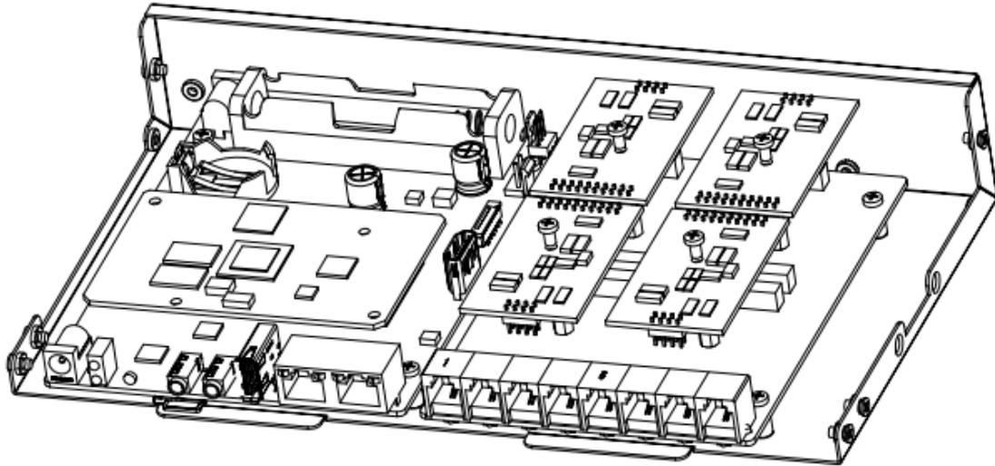
(2) **For old module** : The upper area is for the FXO-100/FXS-100 module and the lower area is for the FXO-400/FXS-400 module. It should be noted that the module cannot be installed on the left or right side at the same time, only supports ①+②, ③+④, ①+④, ②+③. Users can choose two module accessories to customize.
