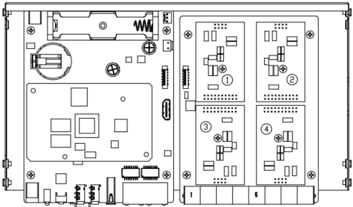
Remove the screw and install the module.
