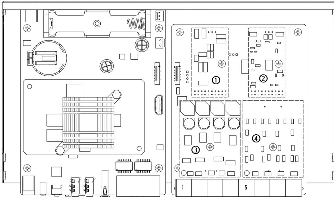
Remove the screw and install the module (②+③) .
